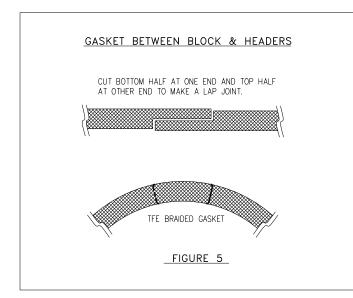
The gasket must be placed close to the inner edge of the gasket surface of the head and on the gasket grooves if any. Some exchangers require two strips of gaskets. Always refer to the assembly drawing for details.
