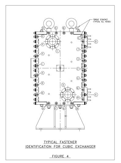
The loosening must be carried out simultaneously by all crewmen. For a team of two, they must alternate from process heads to service heads for each successive nut but each workman must always work on opposing heads.
